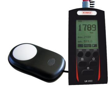
**LX200** hand-held luxmeter, self-contained and automatic is specially designed to illuminance measurement. It allows storage of datasets for processing on a computer via the **LLX200** software.
